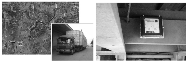
图 2 家电货运卡车与 SAVER 安装位置 Fig. 2 Household appliance freight trucks and SAVER installation position
