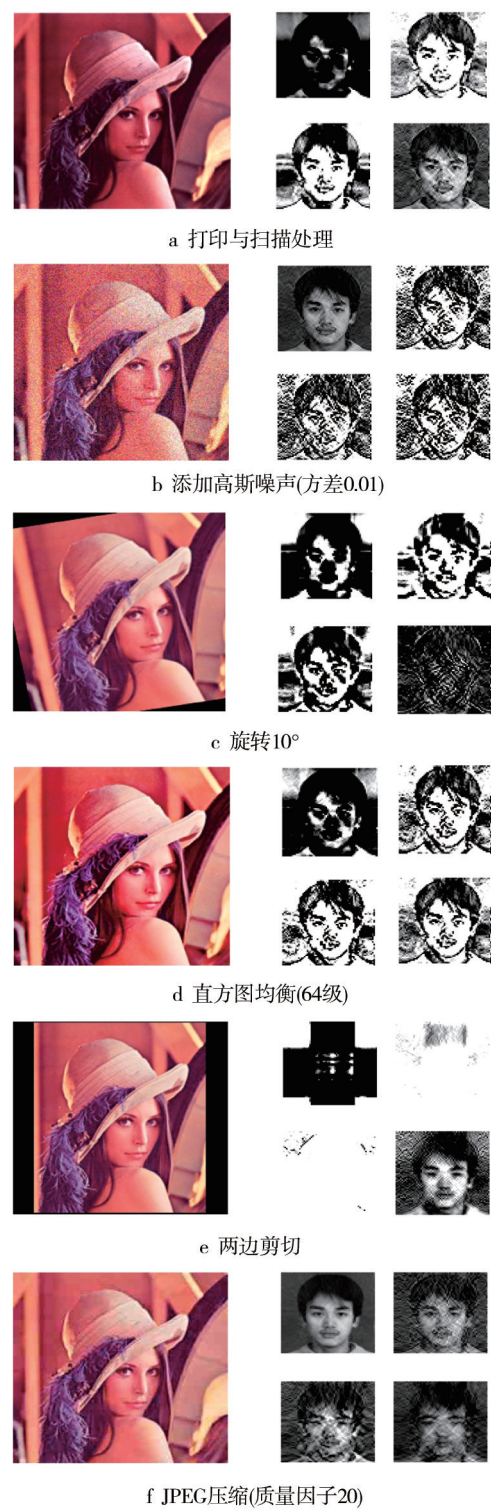
图6 各种攻击后含水印图像及其从4个频带中提取的水印图像 Fig.6 The watermarked image and the watermark image extracted from the 4 frequency bands after all kinds of attacks
