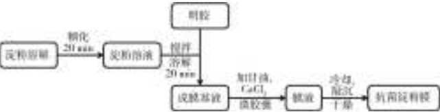
图1 抗菌淀粉膜制备工艺流程 Fig.1 The flow chart of antibacterial starch film preparation process
