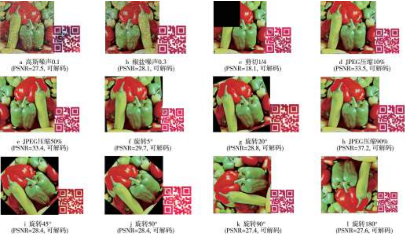
图6 水印鲁棒性仿真实验结果 Fig.6 The simulation results of watermark robustness
