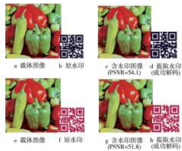
图5 水印嵌入和提取仿真结果 Fig.5 Simulation results of watermark embedding and extracting
