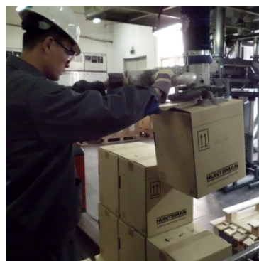
图8 单箱提升 Fig.8 Single box lifting
