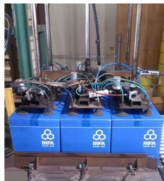
图7 9箱(3×3)整体提升 Fig.7 Overall lifting
