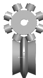
图 5 弧面分度凸轮机构 Fig.5 Globular indexing cam mechanism
