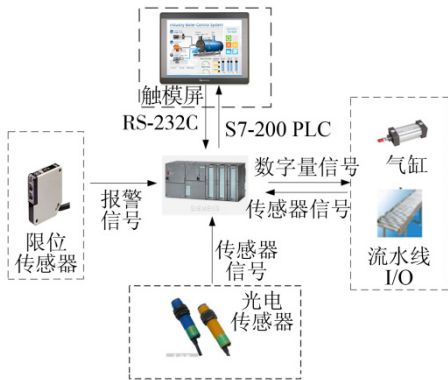
图 2 气动机械手控制系统结构原理 Fig.2 The structure and principle of pneumatic manipulator control system
