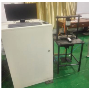
图 5 称量传感器蠕变误差检测试验设备 Fig.5 Test equipment for creep error detection of weighing sensor
