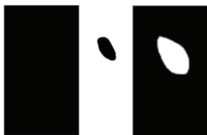
图 8 脱墨和污点缺陷 Fig.8 Void and spot defects
