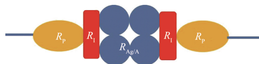
图4 打印电路电阻 Fig.4 Resistance of the printing circuit
