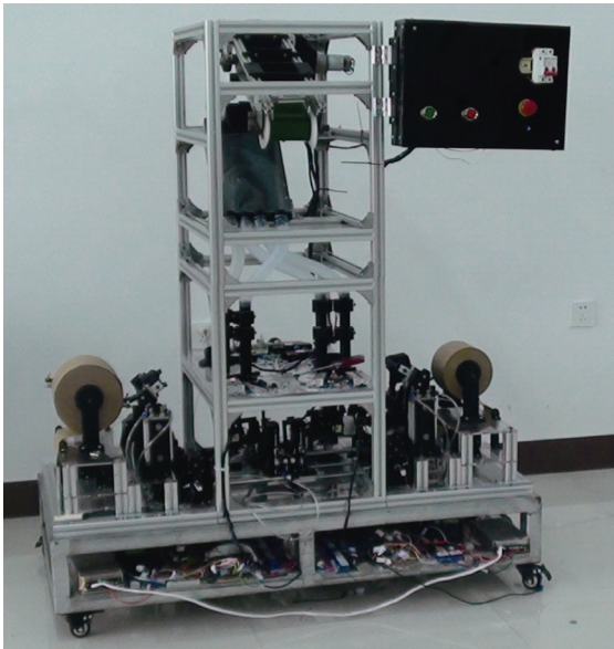
图 9 硬币清分打包机样机 Fig.9 Prototype of automatic belt coin differentiating and wrapping machine
