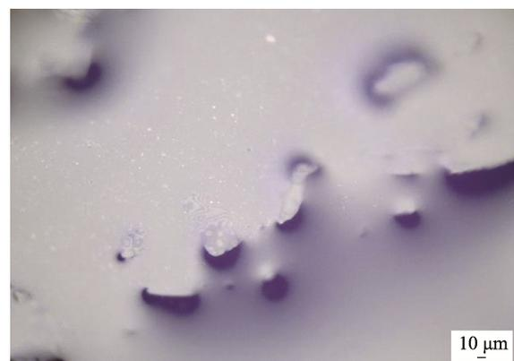
图7 无超声波实验工况下制取海水流化冰晶体 Fig.7 Sea-slurry ice crystals prepared under experiment conditions without aultrasonic wave
