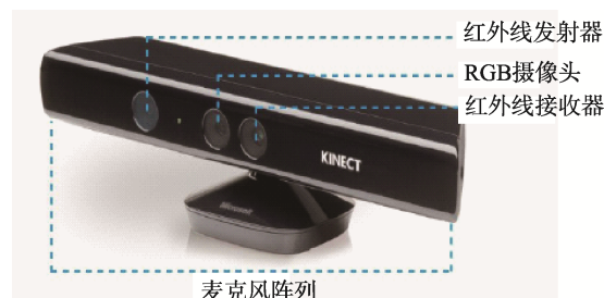
图 1 Kinect 传感器结构 Fig.1 Structure of Kinect sensor
