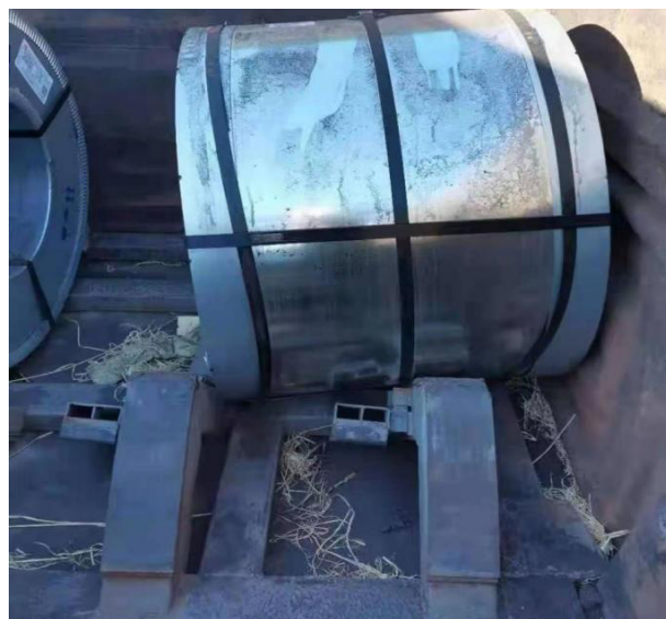
图 1 铁路卷状货物横向位移事故现场 Fig.1 Accident scene of lateral displacement of railway coiled cargo
