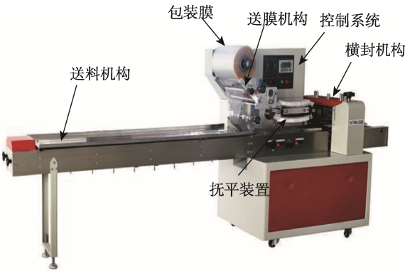
图 1 包装机结构 Fig.1 Structure of packaging machine
