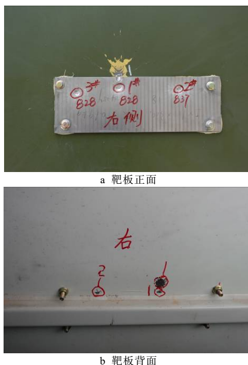
图 7 车辆外部附加装甲实弹测试 Fig.7 Live ammunition test of vehicle external additional armor
