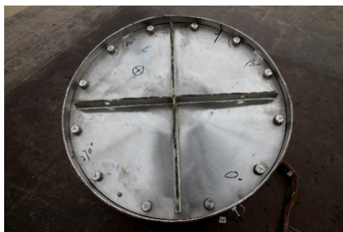
图 5 自由下落试验I顶盖变形结果 Fig.5 Deformation result of head cover under free drop test I
