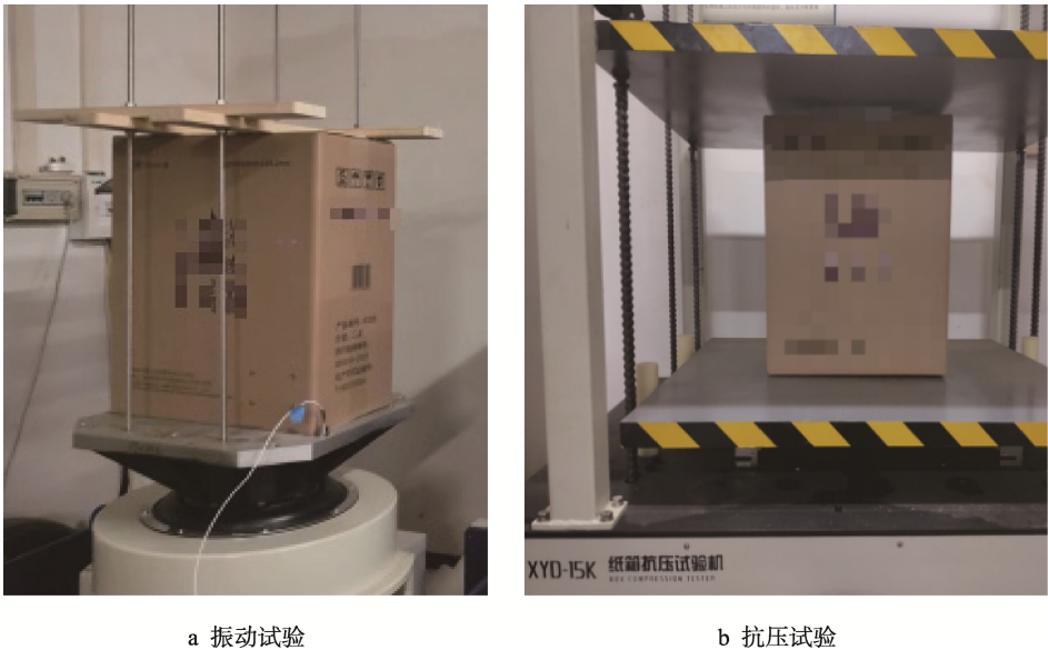
图 6 瓦楞纸箱试验 Fig.6 Corrugated carton test
