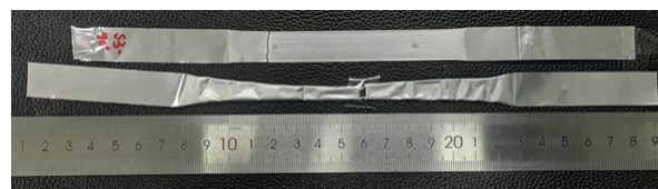
图 4 拉伸断裂后的铝箔和铝塑膜样品 Fig.4 Aluminum foil and aluminum-plastic film samples after tensile fracture
