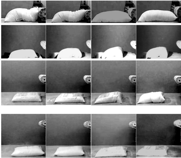
图 14 输送机离地 200、400、600、800 mm 时 不同输送速度的落袋状况 Fig.14 Bag drop condition at different conveying speed when the conveyor is 200, 400, 600 and 800 mm from the ground
