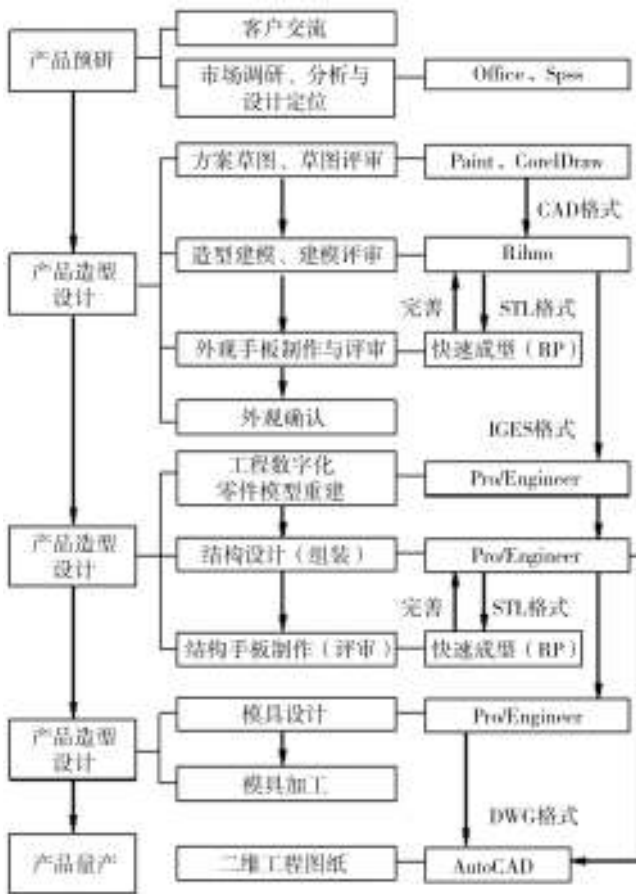
图7 基于设计流程的数字化设计方案 Fig.7 Digital design project based on design process
