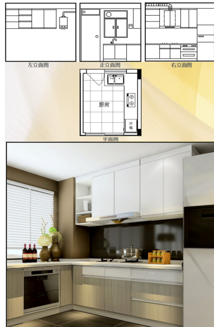
图 3 “尚品宅配”小户型厨房定制家具设计的平面图及三维效果图 Fig.3 The plan and three dimensional effect diagram of custom-made furniture design in small-size house kitchen of "Shangpin Delivery"
