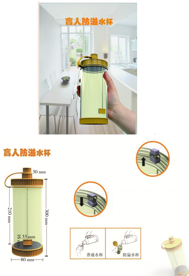
图 3 视障者防溢水杯设计 Fig.3 Blind anti-overflow cup design
