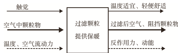
图 11 防雾霾口罩的总功能 Fig.11 Overall function of the antifogging mask
