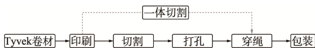
图 11 采用一体式剪裁法的雨衣制作流程 Fig.11 The process of making one-piece raincoat
