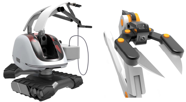
图8 机械臂(手)及视觉装置造型设计 Fig.8 Modeling design of robot arm(manipulator) and visual device
