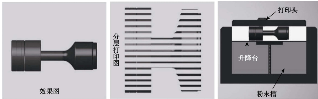
图7 石膏模 3D 打印步骤 Fig.7 The 3D printing procedures of plaster mold
